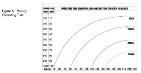
For example, as shown in *FIGURE 6*, using a 400 amp hour battery (batteries), if the average power usage will be 1000 watts, the operating time will be about 150 minutes. A larger capacity battery will deliver more operating time between recharges.
